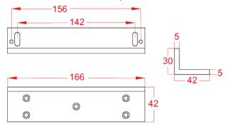
• Z-Brackets for armature plate
