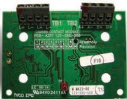
The FC410CIM FC Addressable Contact Input Module is designed to monitor fire contacts such as extinguishing system control, ventilation control, fire door control etc. The FC410CIM can be configured as:
