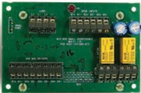
The FC410MIO Multi I/O Module has three inputs and two outputs from latching relays. The inputs can monitor fire contacts such as extinguishing system control, ventilation control, fire door control etc. The two relays outputs provide volt-free relay changeover contacts.
