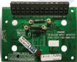
The Addressable FC410DIM provides the ability to connect and Interface one zone of conventional detectors (non-addressable) to the Fire Alarm Controller.
