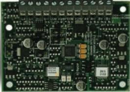
The FC410DDM provides the ability to connect and interface 2 conventional zones, to the FireClass fire alarm controller.
