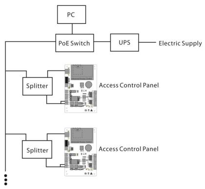
To prevent power failure of a control panel from making the whole system unable to work normally, the access control management system is usually required to have at least one UPS, and access control locks are powered externally to guarantee the access control management system can still work normally during a power failure.
