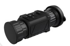
HikMicro THUNDER Pro TQ50C Thermal Monocular has  $640 \times 512$  thermal detector and  $1024 \times 768$  OLED monitor, which provides clear image under harsh environment conditions like darkness, fog, smoke, dust, rain, snow, wood, camouflage, etc. The scope is mainly applied to scenarios such as patrolling, and hunting, etc.
